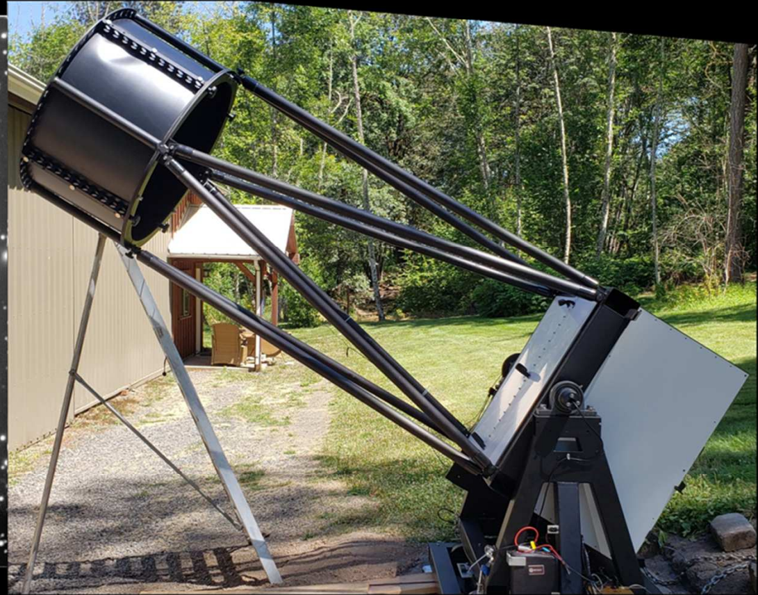
Image from "Jimi Scope" built by Dan Gray & Sidereal Technology team. 36 inch, F4 Alt/Az.
